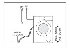
2.Connect it to the branch drain pipe of the trough.
